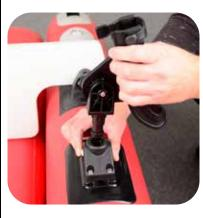
To install a Scotty accessory in the mount, push stem into base until it clicks in. Large knob on side of Rod Holder is for adjusting rod angle.
