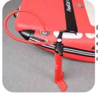
Pump air into the side chambers to give them enough shape to raise the motor mount grommet near to the transom.
