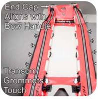
End caps will be centered on bow handles. At the back of the boat, the side motor mount grommets will be touching the inner motor mount grommets.
