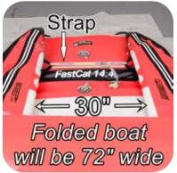
Push the side chambers inward. The boat can be folded without adjusting the width, but the final dimensions will be approximately 82" x 23 x 15. For a more compact fold (72"x 29 x 15), use an 8' strap to pull the bow handles together until there is about 30" between the side chambers.
