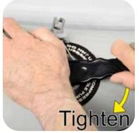
Press on center of valve tool with free hand to keep from breaking the teeth off the tool.
