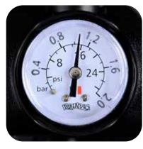
Pressure gauge will not register until chamber begins to get pressurized.
