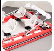
Place the canopy on the back of the boat. Arrange the bars so the long bar is on top and the short bar underneath.
