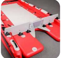
When all transom screws have been inserted, inflate the sides to working pressure.
