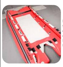
Remove transom, seat frames, rod holders and canopy. Rod holder bases can remain in place in boat. Place the boat bag under front of boat.
