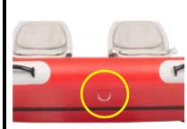
The FastCat14.4 has a large D-ring located under the front chamber. The D-ring can be used as an attachment point for a trailer winch or to hook up to a mooring.
