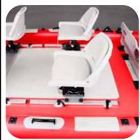
Seat Frame Placement Correct loading of the Fast-Cat14.4 is important for safety, performance, and comfort. Seat frames can be adjusted fore and aft by moving the adjustment knobs. When operating FastCat14.4 without passengers, move the adjustment knobs to the back holes, slide frame forward and strap frame down.
