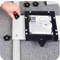
Place a washer on each screw, run screw through the holes in the bar. Place the board over the screws so they are inserted through the board. Secure screw with knob.
