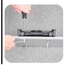
Attach seat mounts to frame board. Place seat mount over the holes in the bench so the screws go through the bench. Place washer and locking nut on the screw. Hold screw with phillips tip screwdriver and tighten nut with 7/16" or adjustable wrench. Aluminum is relatively soft, do not over tighten screws.
