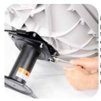
Match up the holes in the pedestal with the holes in the swivel. Insert screws one at a time and hand tighten the locking nuts. When all four screws are installed, use two wrenches to tighten each locking nuts.
