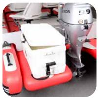
**Cooler (Not included or sold by Sea Eagle)** Two D-rings are installed on the floor aft of the transom for strapping on a cooler or utility box. Cooler should be smaller than 54 gallon capacity and have two handles or slots for strap.
