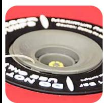
To deflate, push down on the valve stem and quarter turn it to the right or left. The stem will stay in the down position, allowing the air to escape.
