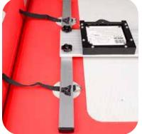
Place frame on the boat. Frame bars go on top of floor hold down straps.
