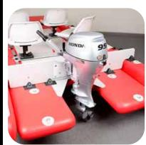
**Motor (OPTIONAL)** Clamp electric motor or up to a 20hp gas motor to motor mount. Turn clamp screws until tight.
