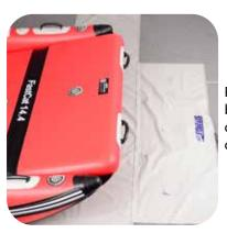
Place boat bag under the bow. Line up bottom panel of boat bag with front edge of the boat.
