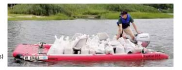
The FastCat14.4 has four floatation chambers; two side chambers and two floor chambers. The boat will stay afloat and can be paddled or motored when loaded to 50% capacity with the main chamber deflated.
